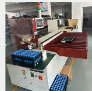
电池配对 Cell Capacity & Voltage Matching
