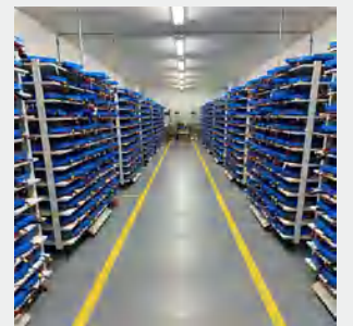
电池测试 Battery Pack Capacity Testing and Aging
