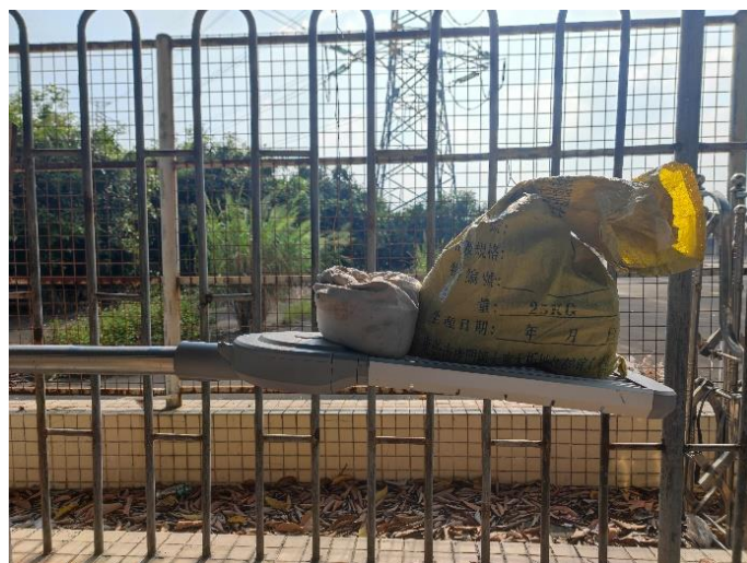
Static load test
