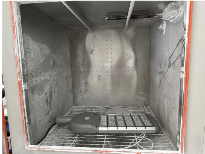
IP6X dust test
